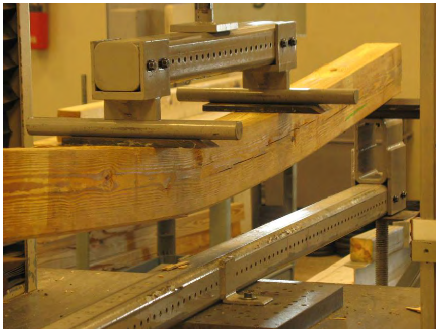
Photo No. 8 TimberSIL Test Series Specimen at Initial Failure Load
