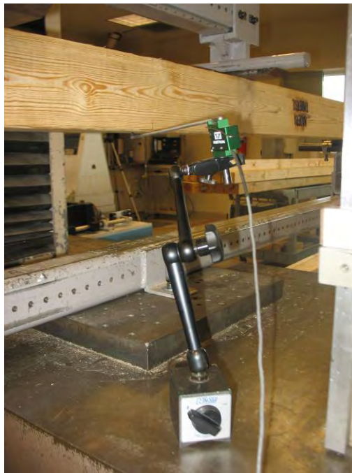
Photo No. 4 Deflection Measurement Apparatus
