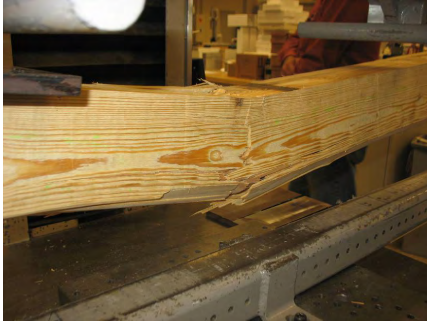
Photo No. 7 Typical Control Series Specimen at Ultimate Failure Condition Detail
