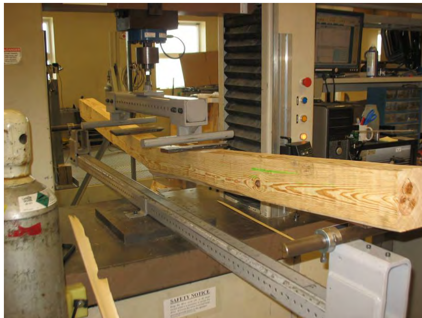
Photo No. 6 Typical Control Series Specimen at Ultimate Failure Condition
