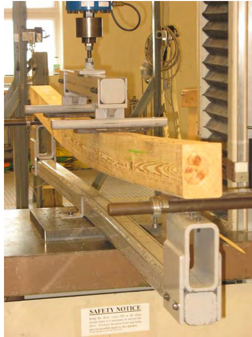
Photo No. 5 Typical Control Series Specimen at Initial Failure Load
