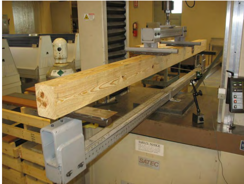
Photo No. 1 Flexural Evaluation Test Setup
