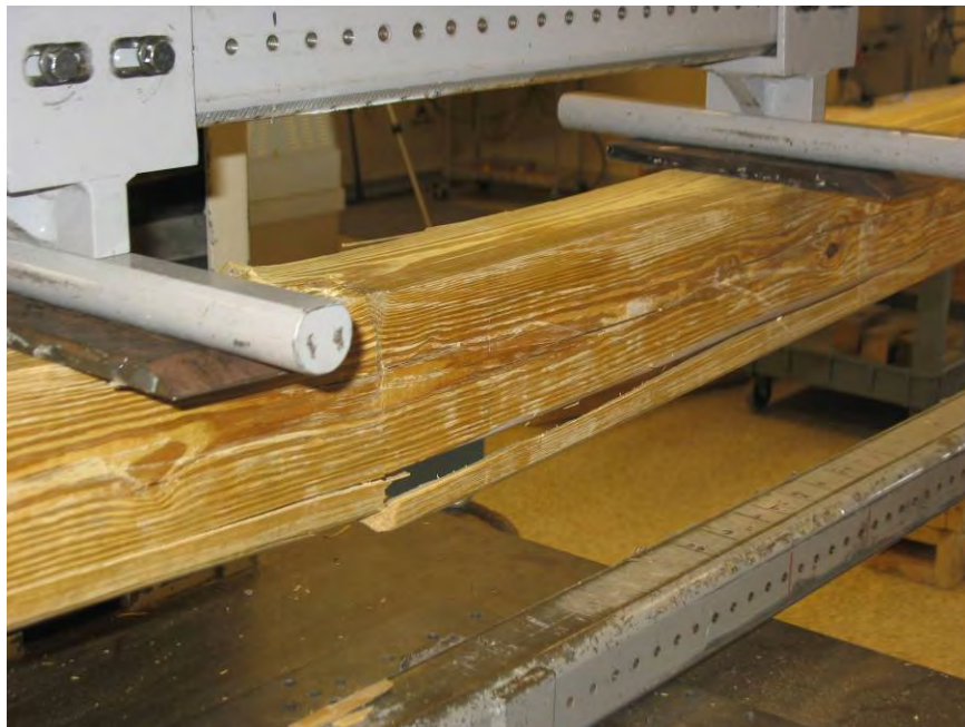
Photo No. 10 TimberSIL Test Series Specimen at Ultimate Failure Condition Detail
